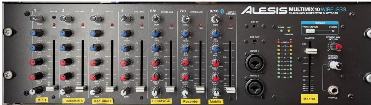
Close to the right side of the Mixer is the master volume control, labelled 'Master'. This is a white slider in a vertical groove which has a printed scale.
