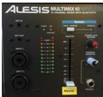
There is also a microphone socket on the Mixer in the Audio Cabinet, labelled Input 1 (see left). This is for using the wired microphone at the back of the hall.
