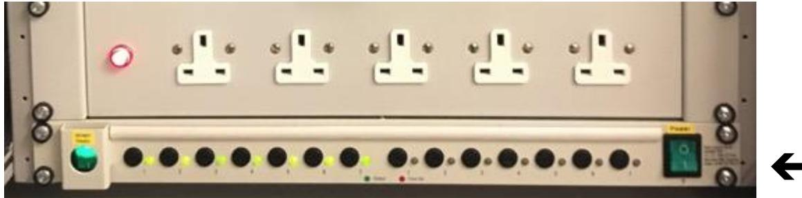
Switch the equipment on using the green rocker switch at the bottom right of the rack.
